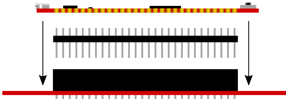
图 2-2. 连接到 Curiosity Nano Base for Click board™
